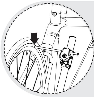
Always take readings with indicator at valve hole to ensure wheel trueness will not impact accuracy of tool. Also, always take readings at outside edge of rim to minimize errors that may be caused by rim's sidewall slope.
