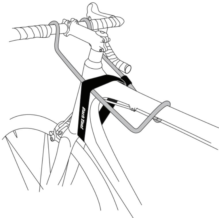
The HBH-2 is designed to prevent the handlebar and front wheel from rotating when the bike is mounted in a Park Tool Repair Stand. Fits bikes with flat and drop handlebars and frame top tubes up to 50mm. Vinyl coated to protect bike finish.
